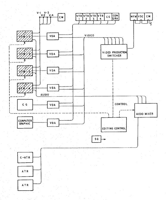
Figure 11.6.2-3 Post Production Block Diagram
