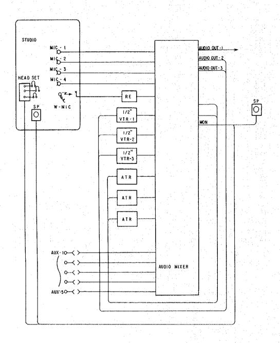
Figure 11.6.1-2 New TV Studio Audio Block Diagram
