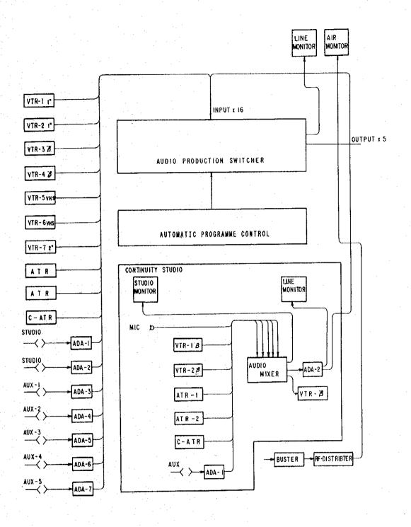
Figure 11.6.2-5 Master Control and Continuity Studio Audio Block Diagram
