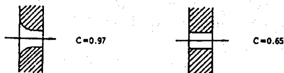
Figure 28 Shape of Orifice and Value of Discharge Coefficient
