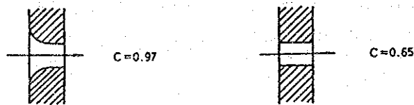
Figure 11.28 Shape of Orifice and Value of Discharge Coefficient
