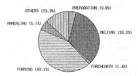
For your reference, a heat balance chart for a medium-sized melting tank in Japan is shown in Figure 8.5. This furnace has a thermal efficiency of about 40 %, and heat loss is mainly from the furnace walls except that about 20 % of the heat is lost in the combustion exhaust gas.
