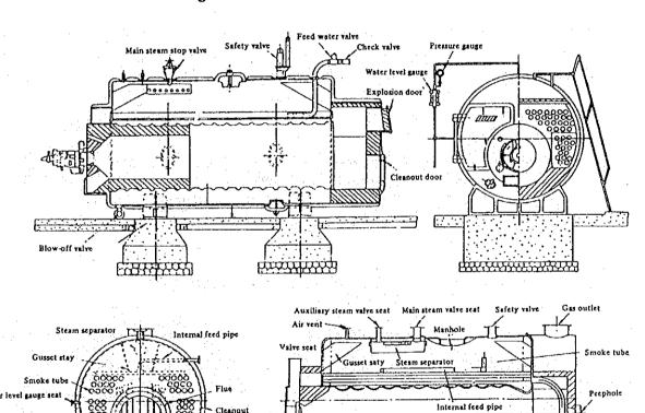
Figure 9.3 Flue Smoke Tube Boiler
