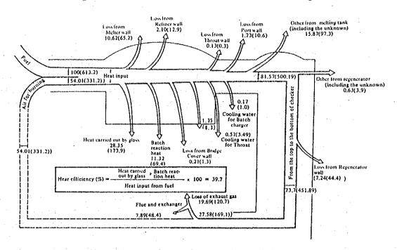
Figure 8.5 Heat Balance Chart for Glass Melting Tank
