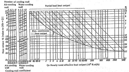
(The figure shows the case that the temperature difference between the heat release surface and the ambient air is 28°C and the wind velocity on the heat release surface is 0.5 m/s. Correction multiples in other condition are based on it of Fig. 9.11.)
