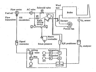
Figure 9.20 Boiler Air Ratio Controller (2)
