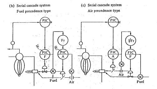
When the fuel component fluctuates, there are some cases in which air flow is controlled more exactly through transmitting the signal to the controller from the  $O_2$  analyzer in exhaust gas.
