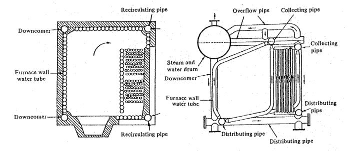
Figure 9.4 Bending Water Tube Boiler
