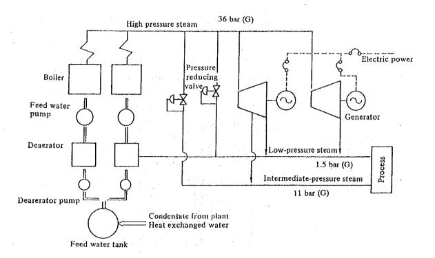
Figure 9.12 An Example of Cogeneration System
