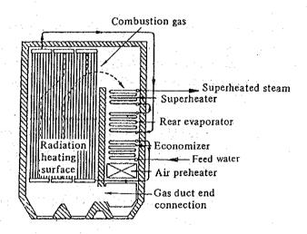
The features of this one-through boiler are as follows:
