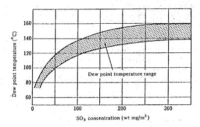
To avoid this trouble, some heat exchangers are used with a glass tube or a lead coating tube as the material. As shown in Figure 9.7 of paragraph of the heat balance, a measure to prevent overdropping of the gas side temperature of heat transfer surface may sometimes be taken by means of preheating the air with an external heat source prior to feeding the air to the air preheater.
