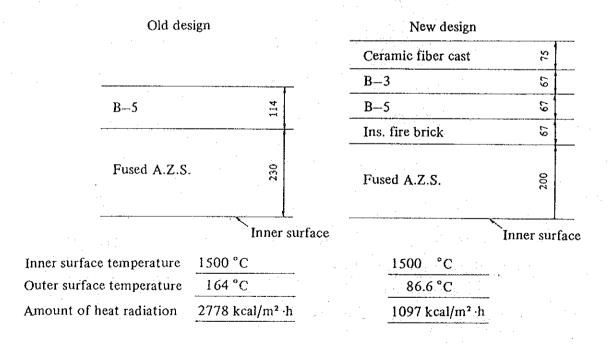
Figure 8.11 Heat Insulation of Regenerator Sidewalls (Upper Part)
