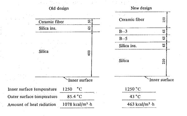
Figure 8.9 Heat Insulation of Regenerator Crown
