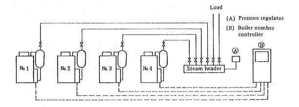
Figure 9.15 Boiler Efficiency Improvement by Operation Number Control
