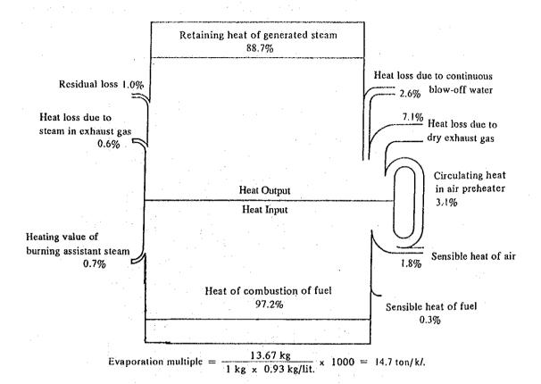
Figure 9.17 Example of 20 T/H Boller Heat Balance
