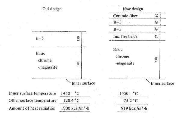
Figure 8.10 Heat Insulation of Port Crown
