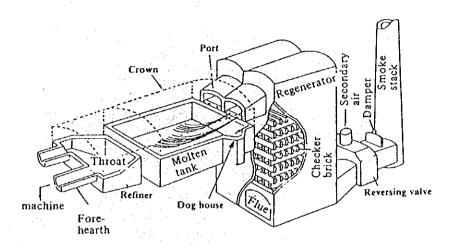
A high temperature of about 1,500 °C is necessary to melt glass so that combustion air must be preheated by heat exchange with combustion exhaust gas. A regenerator or recuperator such as shown in the figure is used for this preheating. Instead of heating with fuel, or as a complementary means, an electrode may be directly inserted into molten glass to directly heat it with electricity.
