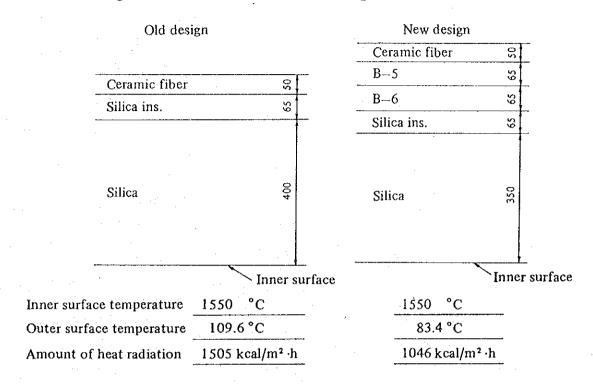
Figure 8.8 Heat Insulation of Working Hearth Crown
