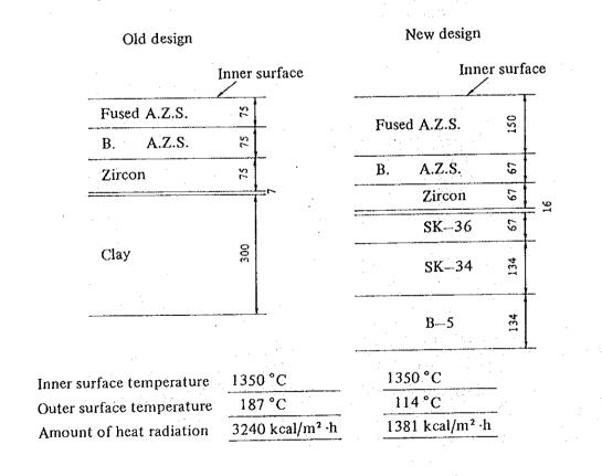
Figure 8.15 Heat Insulation of Working Hearth Bottom
