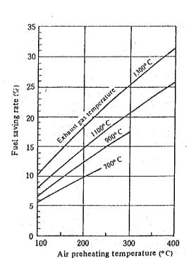
Figure 9.28 Fuel Saving Rate due to Air Preheating
