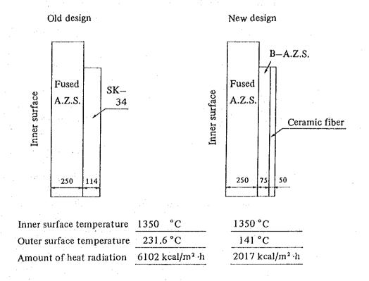
Figure 8.13 Heat Insulation of Working Hearth Tank Block
