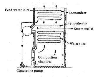
A one-through boiler only composed of a series of long water tubes is designed so that feed water is pushed into the tube by a pump from the end of the tube, by turn temperature is raised, evaporated, superheated and taken out as superheated steam from another end of the tube. Accordingly boiler water is not circulated (see Figure 9.6).
