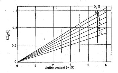
Figure 9.26 Relation between Sulfur Content in Fuel and Conversion Ratio from SO<sub>2</sub> to SO<sub>3</sub>
