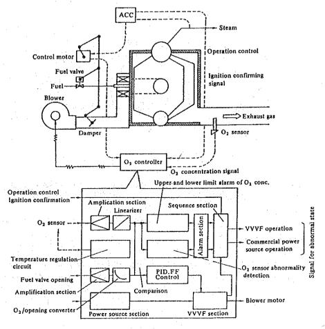
Figure 9.21 Basic Combustion Control System
