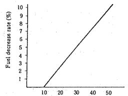
Consumption rate for cullet (against the weight of finished product) (%) Based on the consumption percentage of 10% for cullet.
