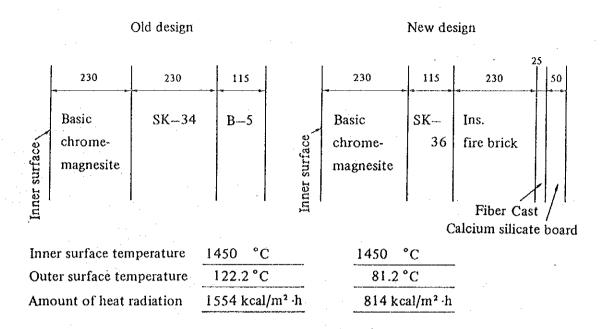
Figure 8.12 Heat Insulation of Melting Tank Block
