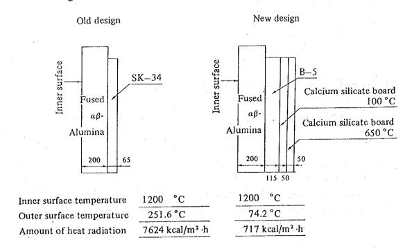
Figure 8.14 Heat Insulation of Melting Tank Bottom
