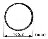
Steel pipe: Dia. 165.2 (mm) x Thickness 5 (mm)
