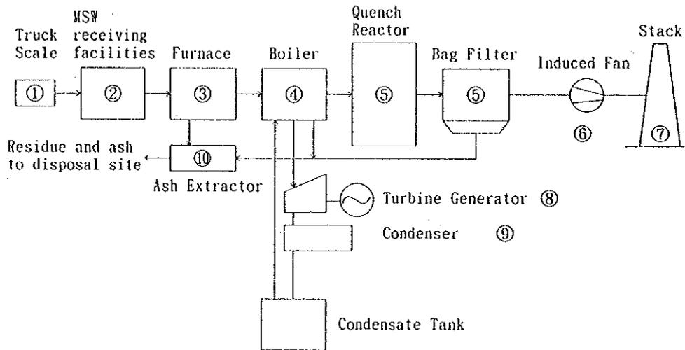
Figure 5-3 Process Flow
