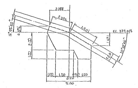
Only the weight of steel pipe and water in the pipe directly above the anchor block is considered.
