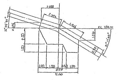
Only the weight of steel pipe and water in the pipe directly above the anchor block is considered.
