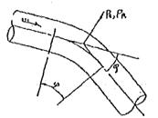
iii) Thrust Due to Internal Pressure
