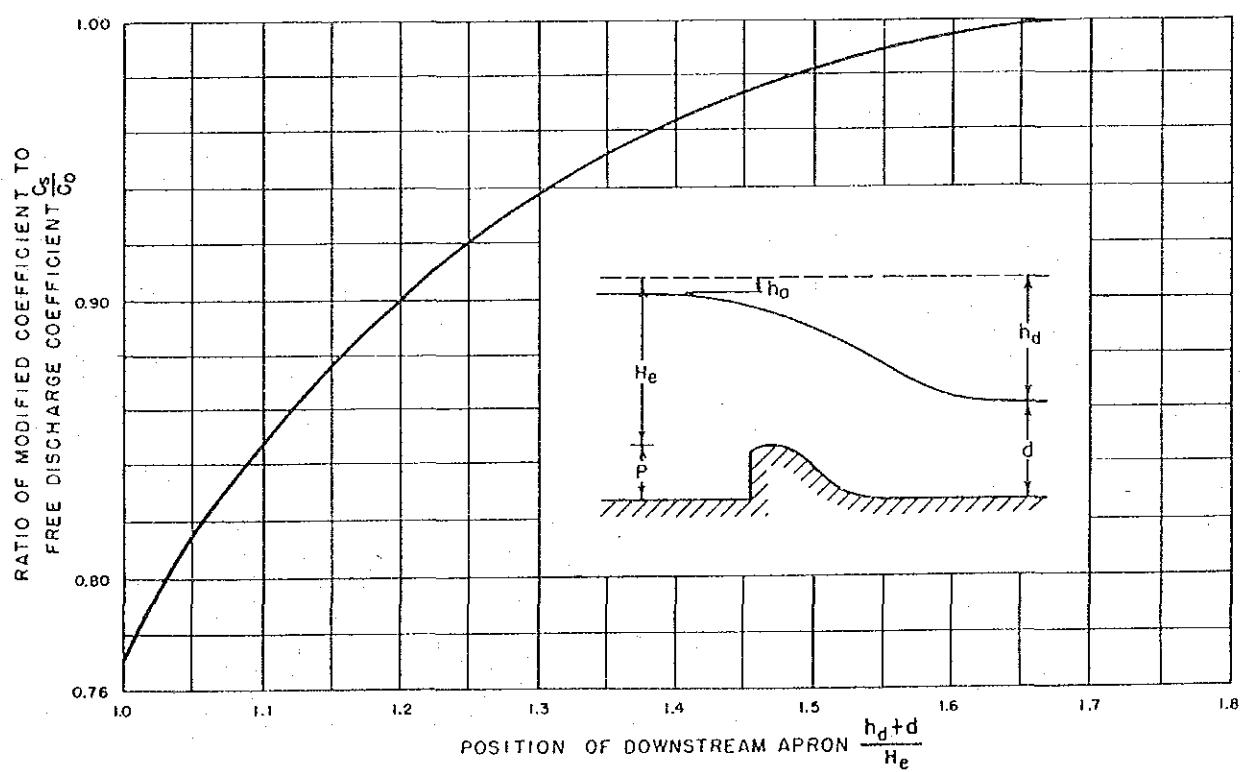
Fig. 5 Ratio of Discharge Coefficients Resulting from Apron Effects
