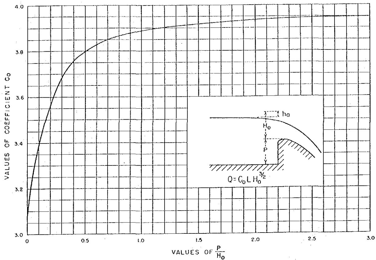
Fig. 4 Discharge Coefficients for Vertical-faced Ogee Crest
