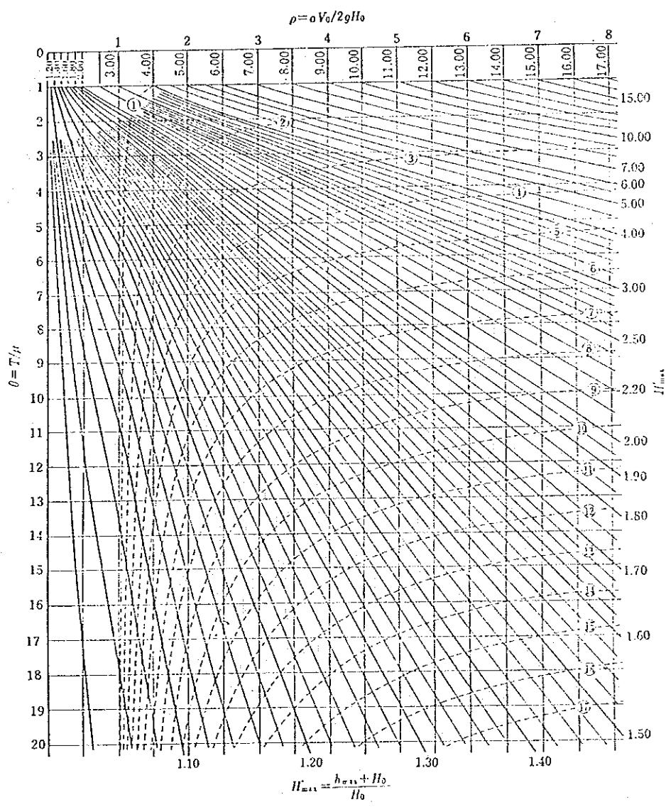
**Fig. 6 Maximum Pressure Rise in Pnstock**
