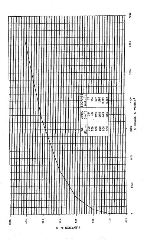
Figure 6.2.4 Storage-Volume Curve for D/S Dam Axis (Axis-II)
