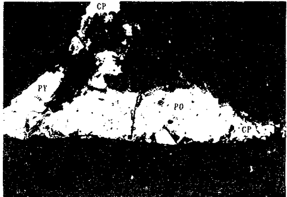
SAMPLE NUMBER: SPOT-01 LOCALITY: SPOT MINE REMARKS: Pyrrhotite-pyrite-chalcopyrite association
