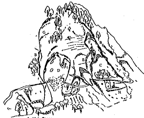
A : Main Scarp B : Crack on Side Flank C : Previously Occurred Landslide of Left Side D : Previously Occurred Landslide of Right Side E : Scarp Trace of Previously Occurred Landslide of Left Side F : Small Scale Landslide occurred at Behind Slope G : Tension Crack in Landslide Area H : Road Destroyed in Left Side Landslide I : Road Destroyed in Right Side Landslide
