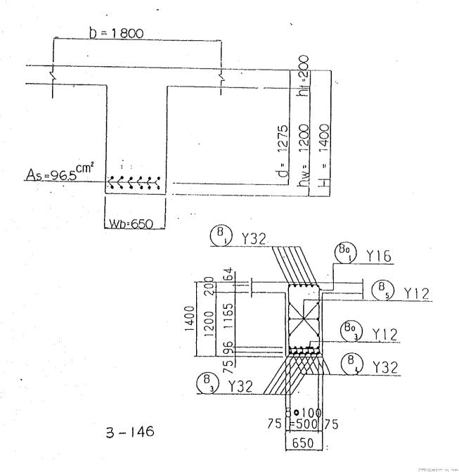
Calculation of deck slab for Main bridge
