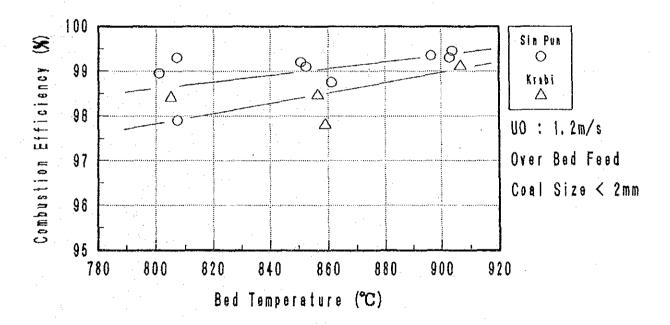
Fig 8-43 Combustion efficiency with different bed temperatures
