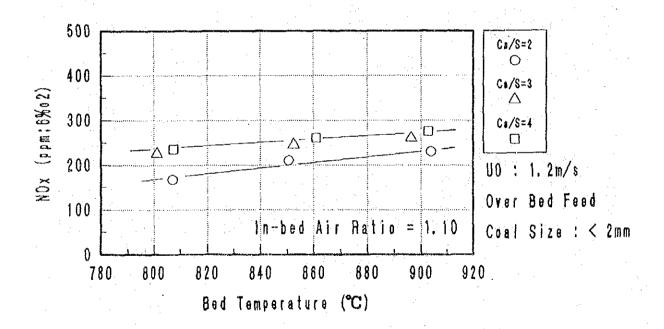
Fig 8-36 NOx emission with different bed temperatures
