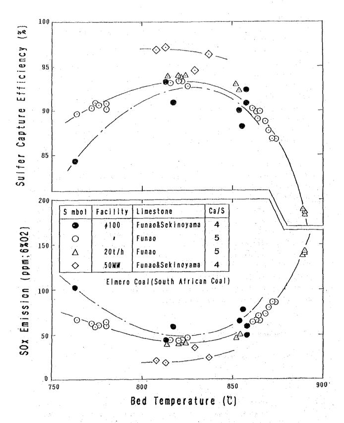
Fig 8-45 Desulfurization characteristic with different scale
