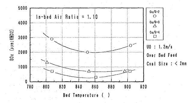
Fig 8-34 SOx emission with different bed temperatures and Ca/S molar ratio
