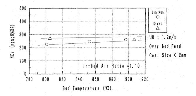
Fig 8-42 NOx emission with different bed temperatures
