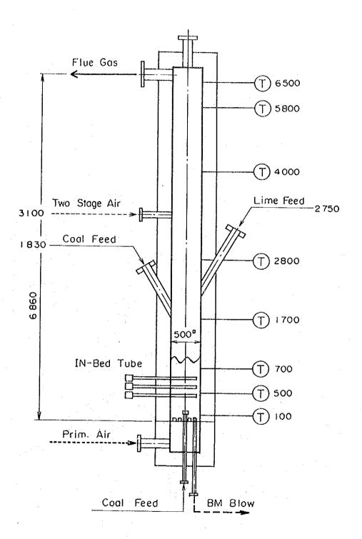
Fig. 9-3a Combustion Test Furnace
