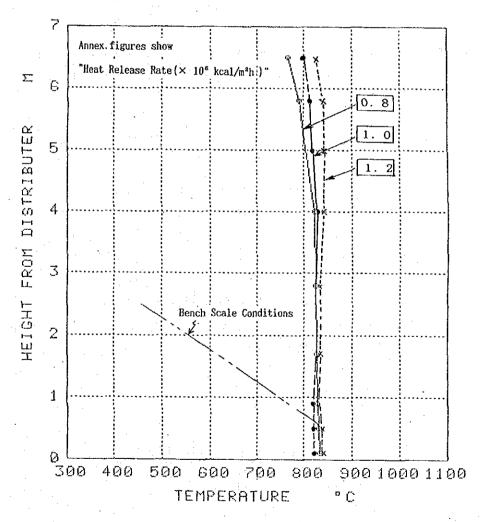
Fig. 9-7 Temperature Profile (Effect of Heat Release Rate)
