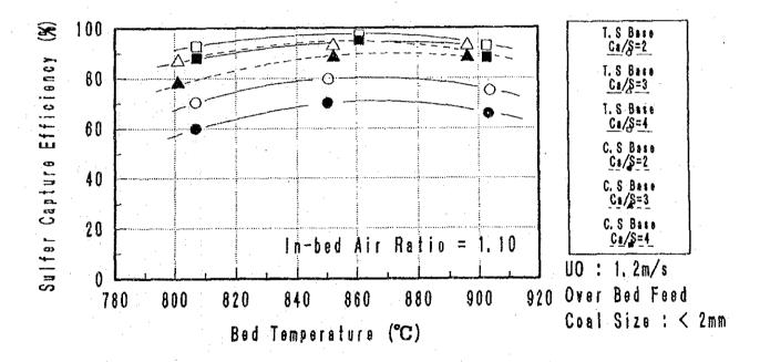
Fig 8-35 Sulfur capture efficiency with different bed temperatures and Ca/S molar ratio
