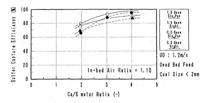
Fig 8-41 Sulfur capture efficiency with different Ca/S molar ratios
