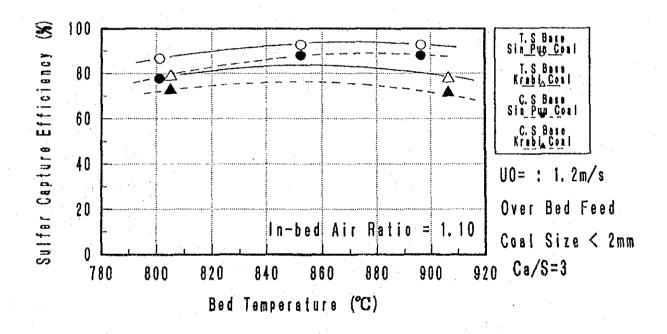
Fig 8-39 Sulfur capture efficiency with different bed temperatures
