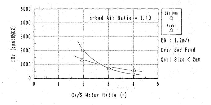
Fig 8-40 SOx emission with different Ca/S molar ratios
