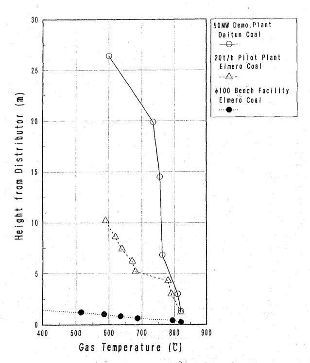
Fig 8-47 Gas temperature distribution in furnace
