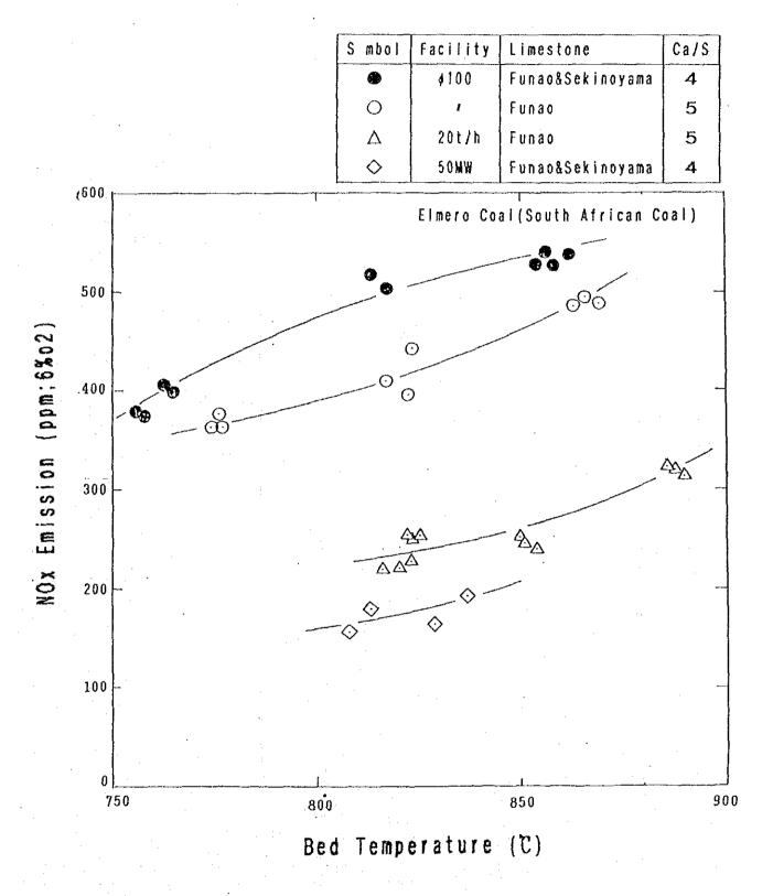
Fig 8-46 NOx emission characteristic with different scale
