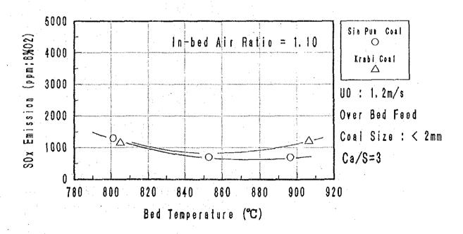
Fig 8-38 SOx emission with different bed temperatures
