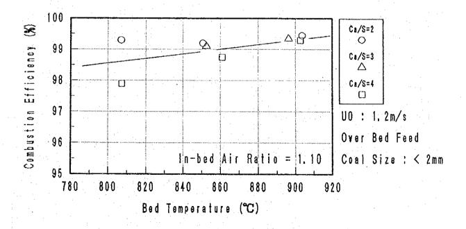
Fig 8-37 Combustion efficiency with different bed temperatures
