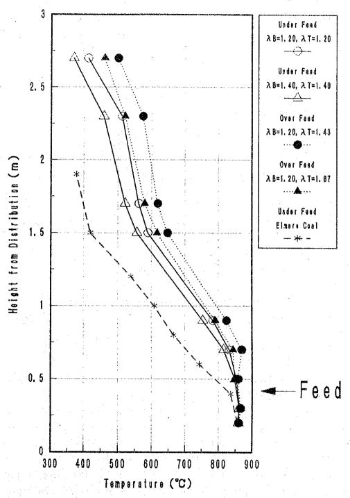
Fig 8-53 Gas temperature distribution in furnace
