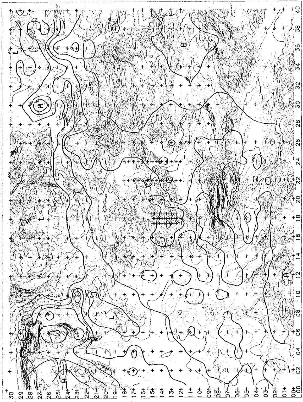
Fig. II-3-11 Resistivity image at the 1050m level
