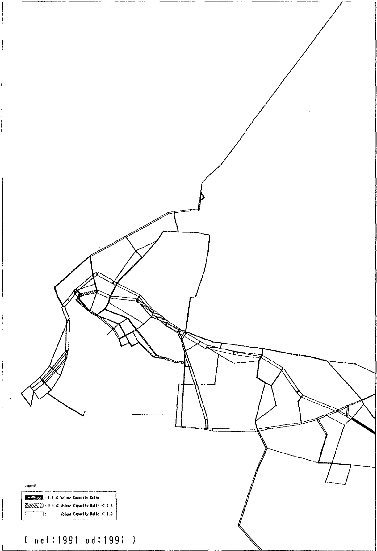
Figure 7.4-11 Traffic Demand in 1991 on the Present Network
