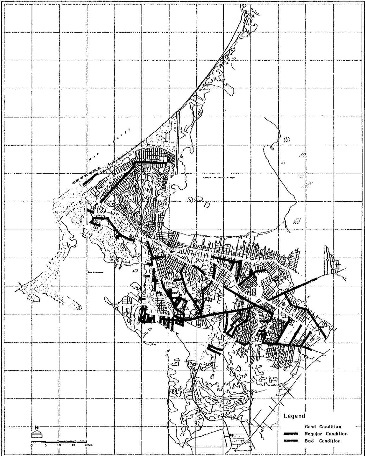
Figure 3.2-4 Pavement Conditions on Roads in the Urban Area
