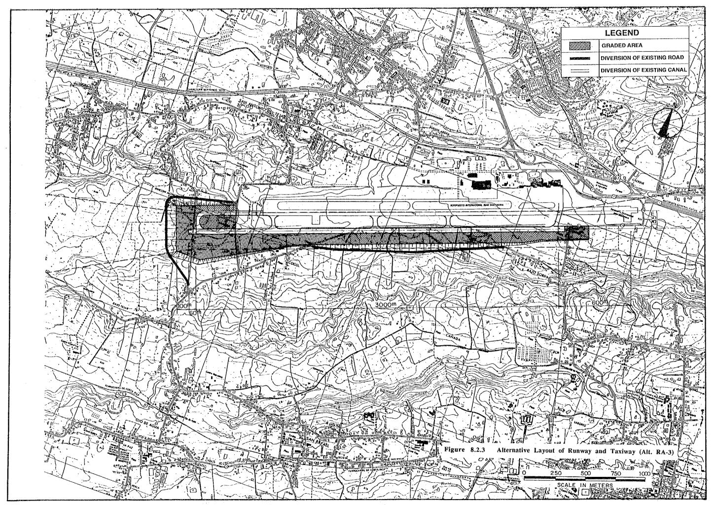
Alt. R-B1 (Continuous use of existing runway with taxiway improvement measures 1 plus 2 - addition of parallel taxiway to Runway 25 threshold and improvement of existing western section of parallel taxiway for use of wide-body jets: Figure 8.2.4)
