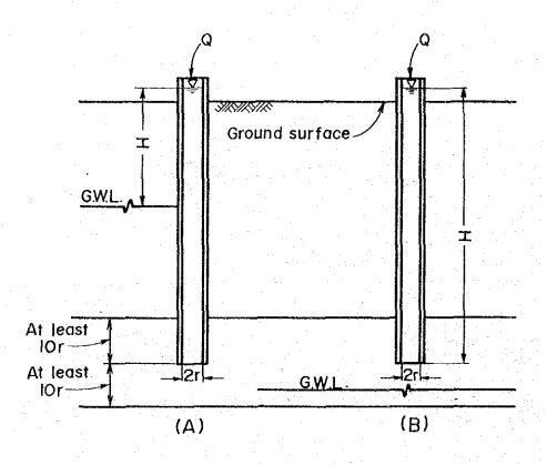
Fig. II .1.7 Open-End Test
