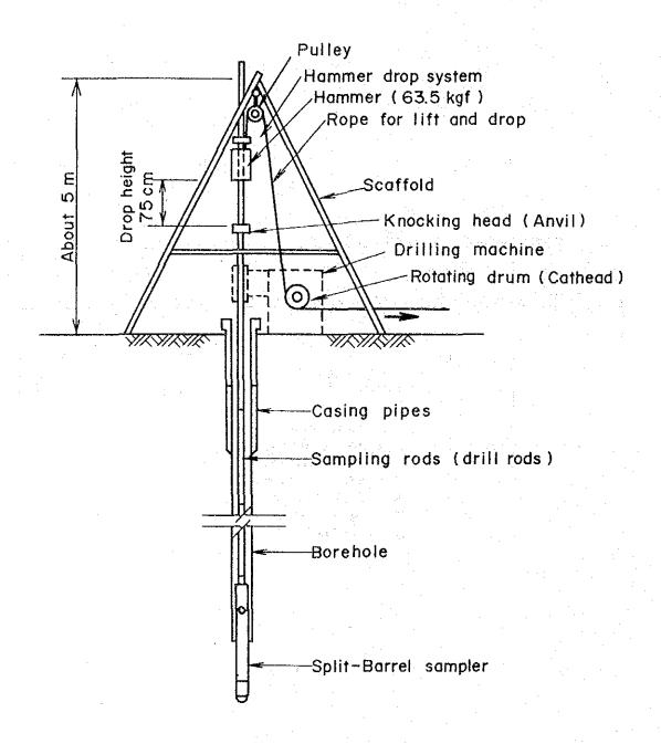
Fig. II.1.3 Standard Penetration Test System
