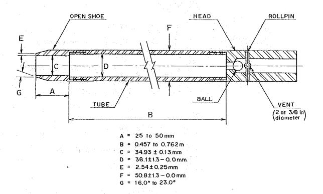
Fig. II.1.2 Split-Barrel Sampler (From ASTM Standards D1586-84)
