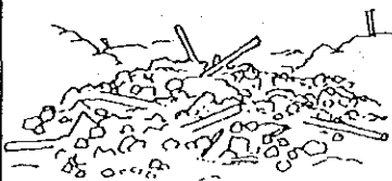
No Structural Elements Distinguishable
