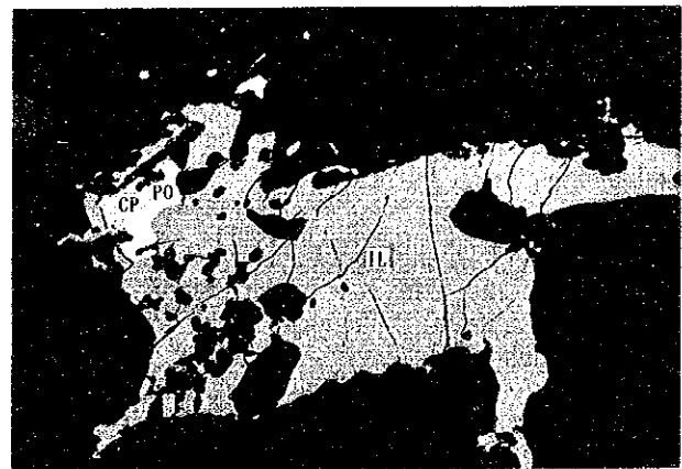
SAMPLE NUMBER : P-08-02 LOCATION : MJZM-08, 140.00 m REMARKS : Ilmenite-Pyrrhotite-Chalcopyrite association
