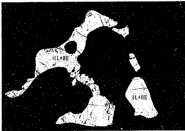
SAMPLE NUMBER : P-03-01 LOCATION : MJZM-03, 7.00 m REMARKS : Exsolution texture of Ilmenite and Hematite
