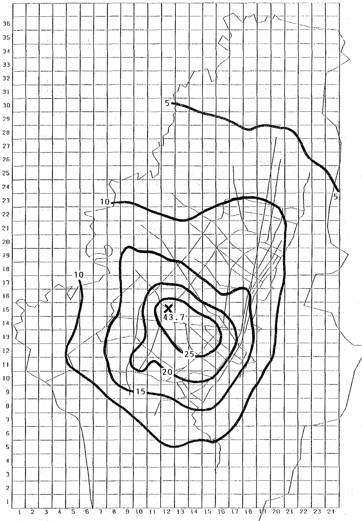
Fig. 7.2.4 Average Concentration Isoleths for SO 2 (All Sources)
