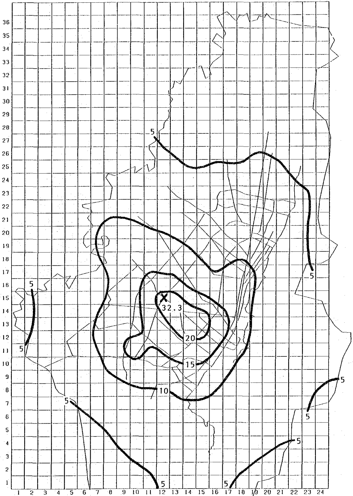
Fig. 6.3.4 Average Concentration Isopleths for SO 2 (All Sources)
