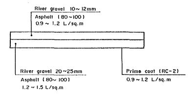
Figure 3.3 Road Structure of Existing Route No.10
