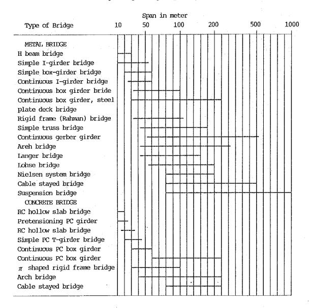
Figure 6.5 Normal Range of Span Length by Bridge Type
