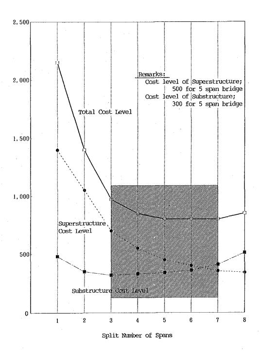
Figure 6.4 Level of Cost by Split Number of Spans
