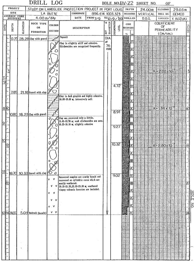
★ RULD in Rock Quality Designation, RULD ~ (Total length of cylindric cores longer than 10 cm)/(Total core length) × 100% #LUCEON VALUE in 1/min/m under injection water pressure of 10kg/cm<sup>2</sup> ★ DEPTH and ELEVATION are in meter
