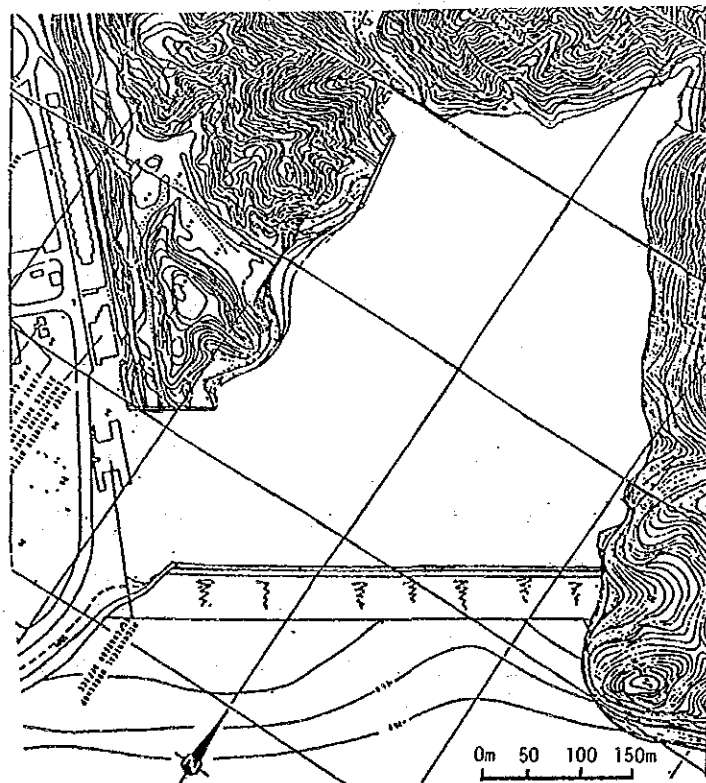
Fig. 8-3-2(B) Land Reclaimed with the Materials Dredged in the -13m Area
