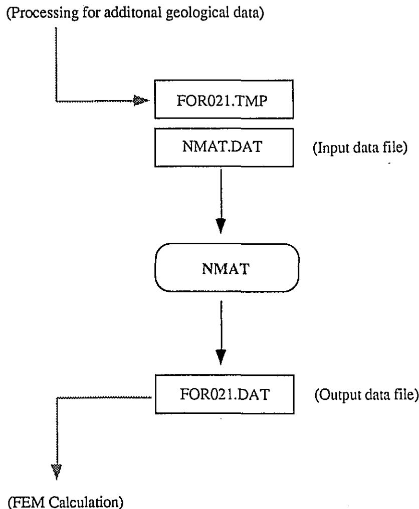
Fig. 13 Processing for Various Symbols of Layer
