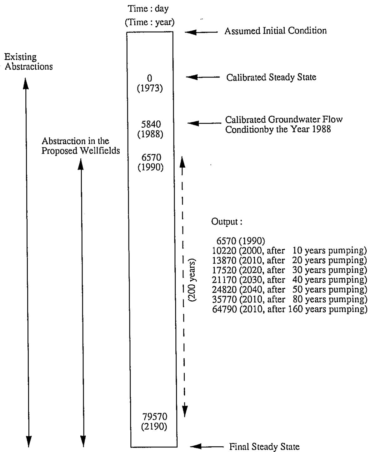
Fig. 28 Procedure of Calculation in Model Simulation
