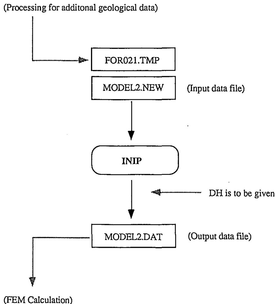
Fig. 17 Processing for Assumption of Initial Head
