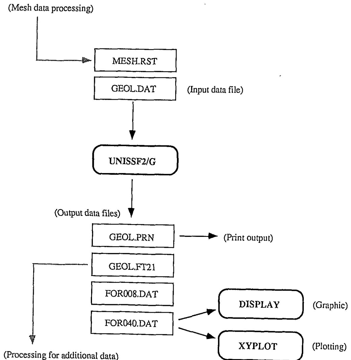
Fig. 5 Geological Data Processing
