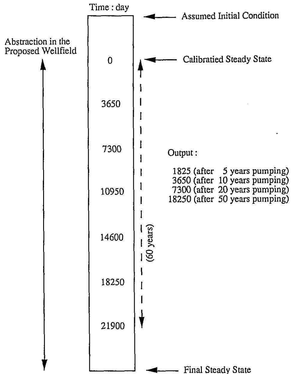
Fig. 22 Procedure of Calculation in Model Simulation
