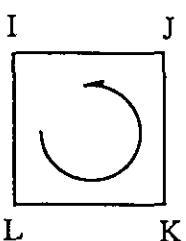
Node numbers of element are given counter-clockwise
