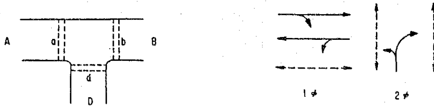
Figure 3.20 2 Phase Arrangement for T-Junction
