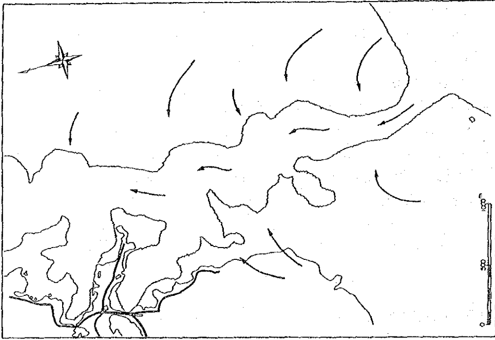
Fig. 5-2 (1) Current Pattern (in flood tide)
