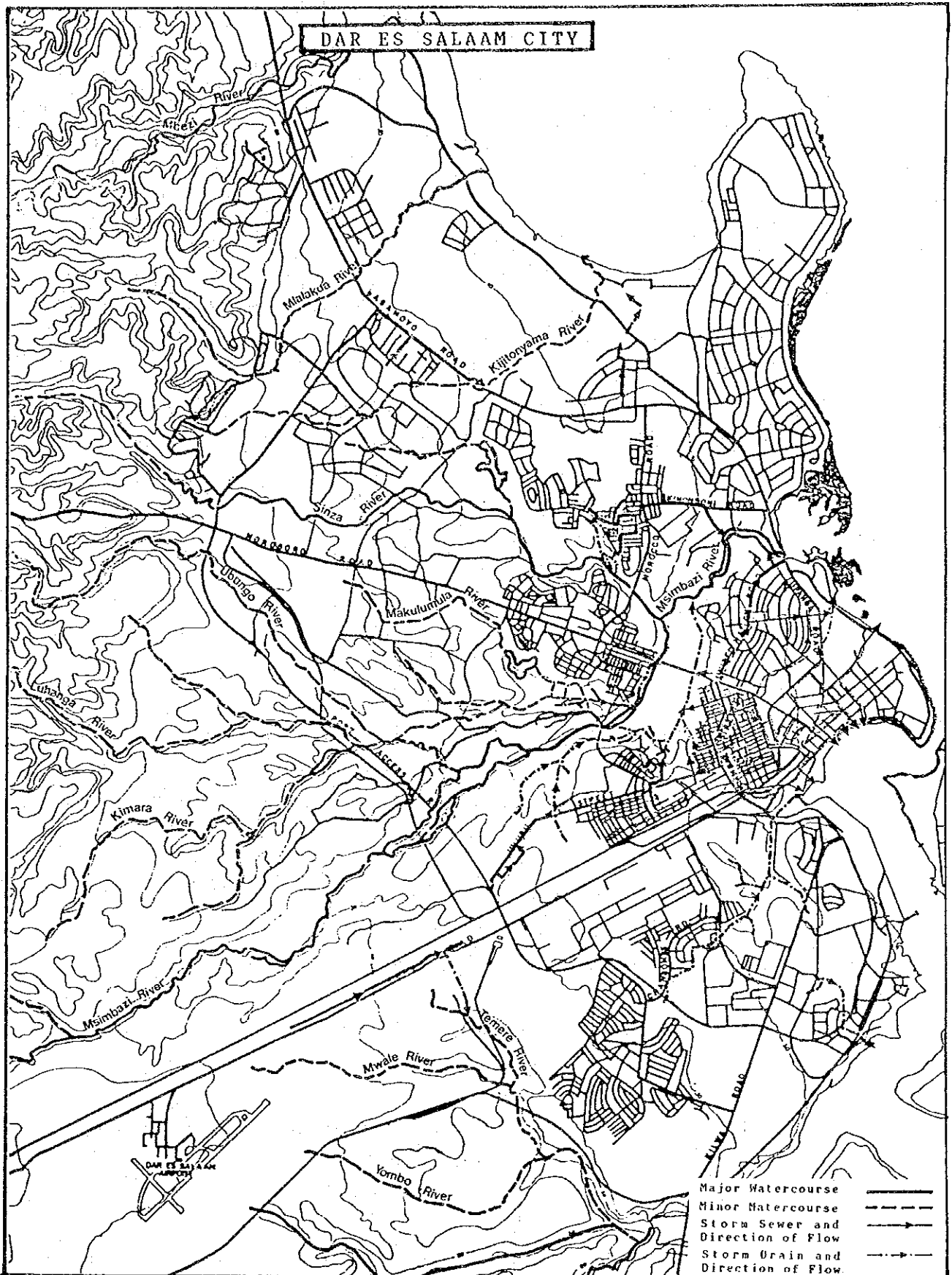
Fig.7.1 Existing Storm Drainage System
