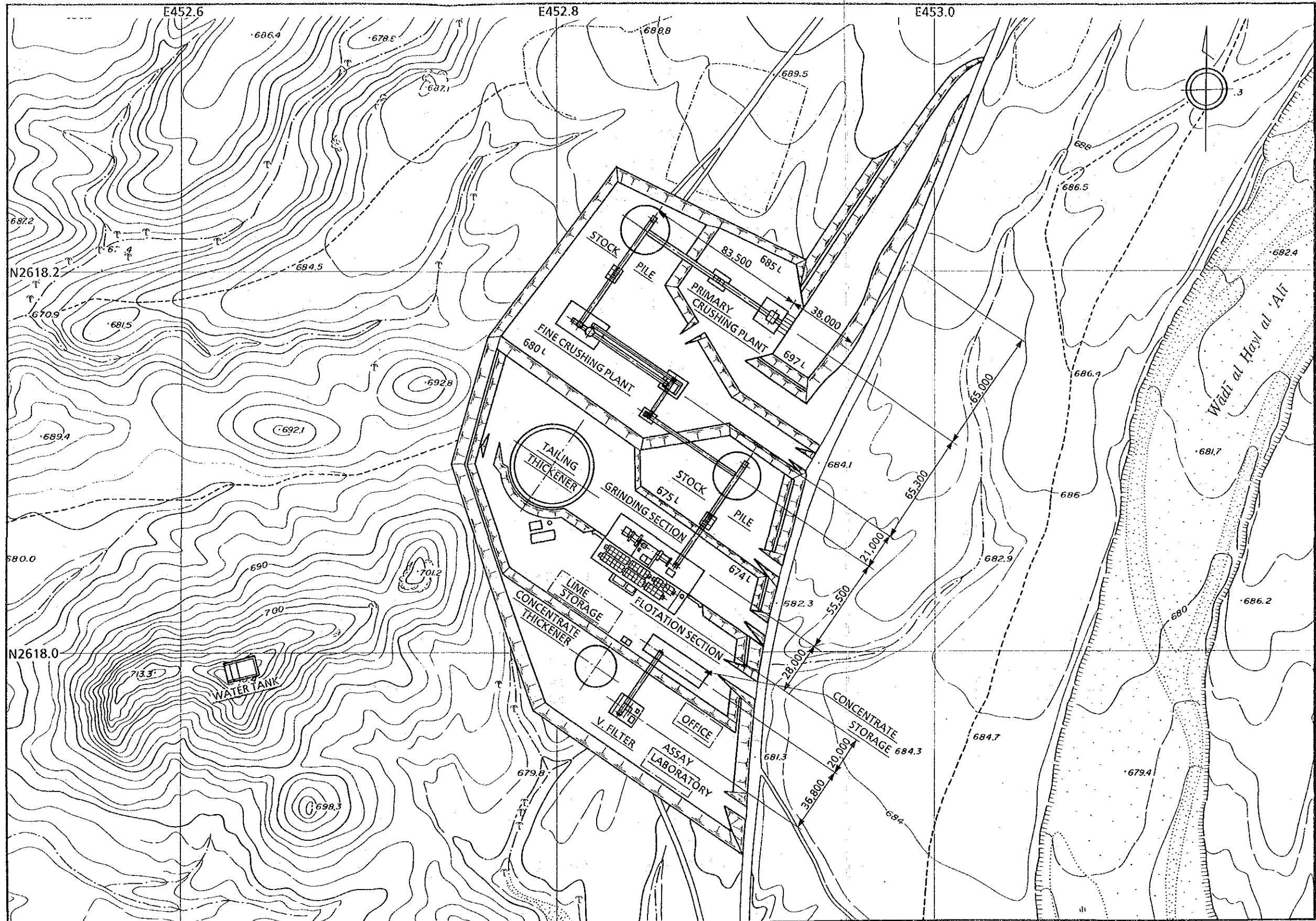
Fig.1 General layout of mineral processing plant
