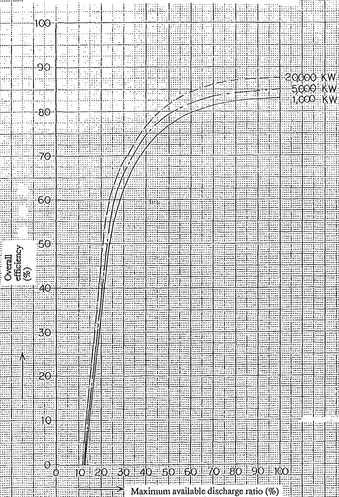
Fig. 8.2 Resultant Efficiency Curve of Pelton Turbine and Generator
