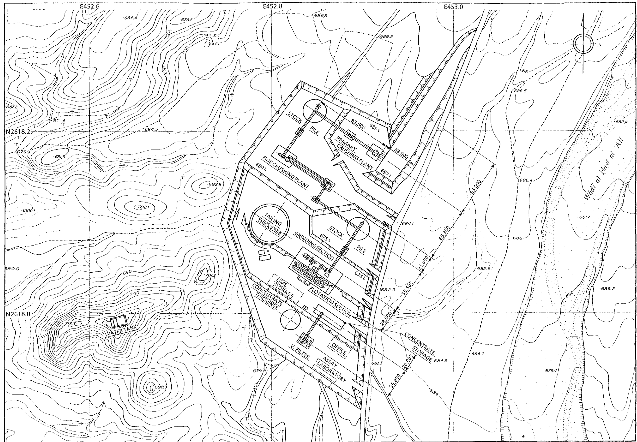
Fig.1 General layout of mineral processing plant
