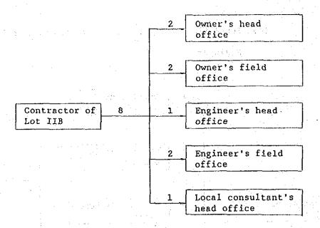
(4) The asbuilt drawings shall be routed as shown below.
