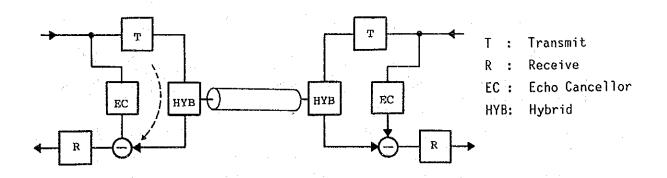
Fig. 7.6 Two-Wire Full Duplex Subscriber Transmission Systems
