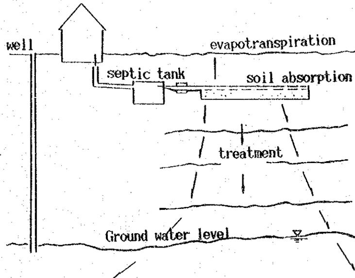
Fig.S8.A.1 Septic tank and soil adsorption system
