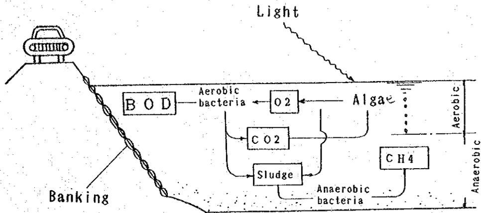
Fig. S8.A.6 System component of Oxidation Pond
