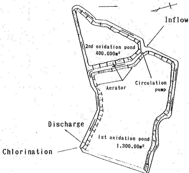
Fig. S8.A.8 Oxidation Pond at Sunnyvale treatment plant
