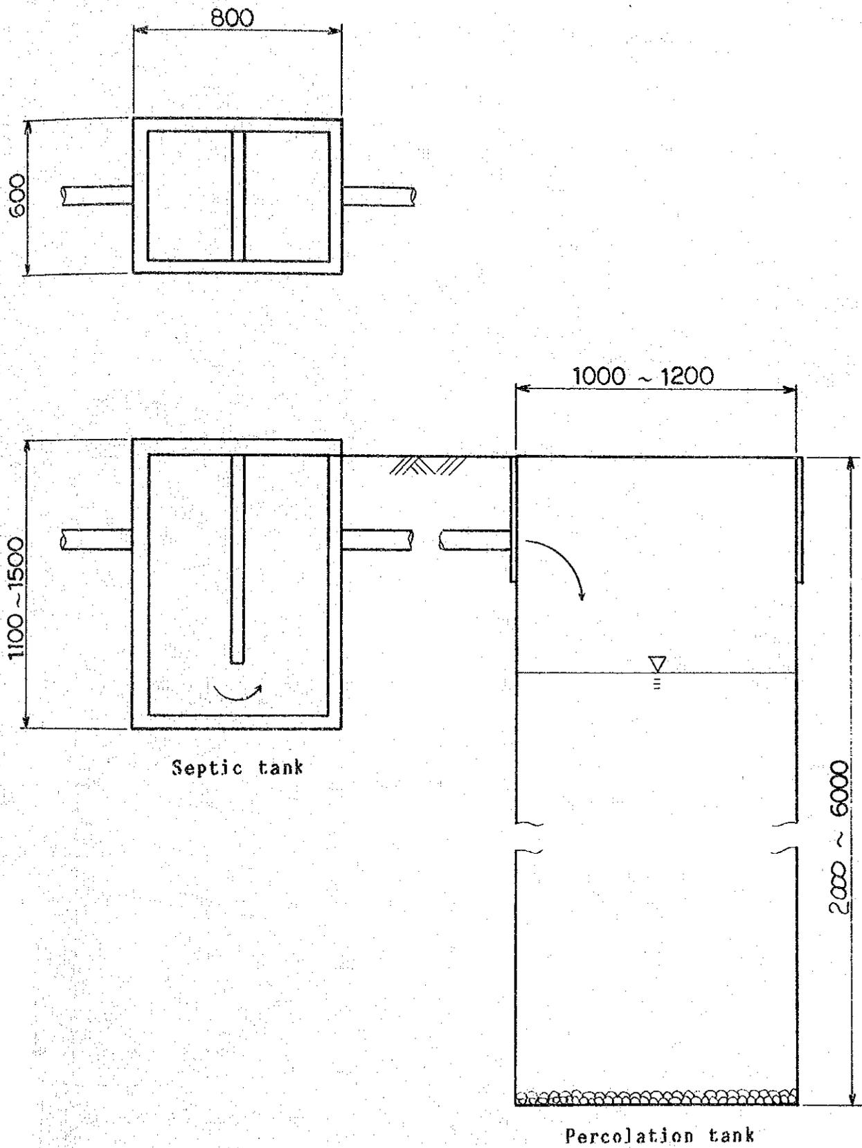
Fig.S8.1.1 Domestic waste water treatment method
