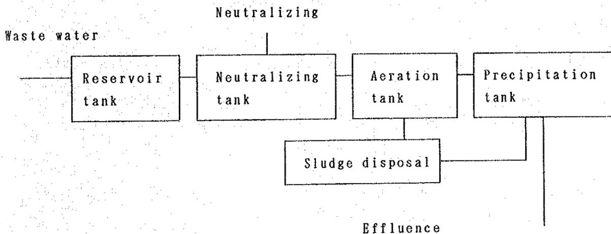
Fig. S8.5.3 One treatment method for Alcohol Facilities
