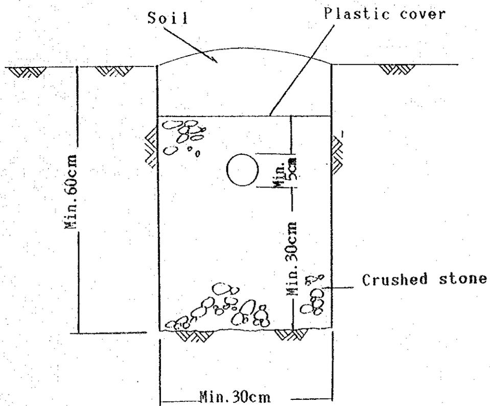
Fig. S8.A.3 section of trench adsorption
