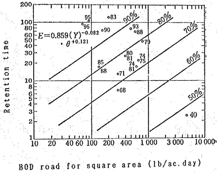
Fig. S8.A.9 Relationship between retention time and BOD removal ratio for canning industrial waste water
