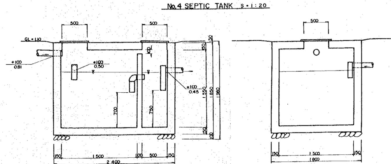
Fig S8. 3.1 Septic tank and soil absorption system
