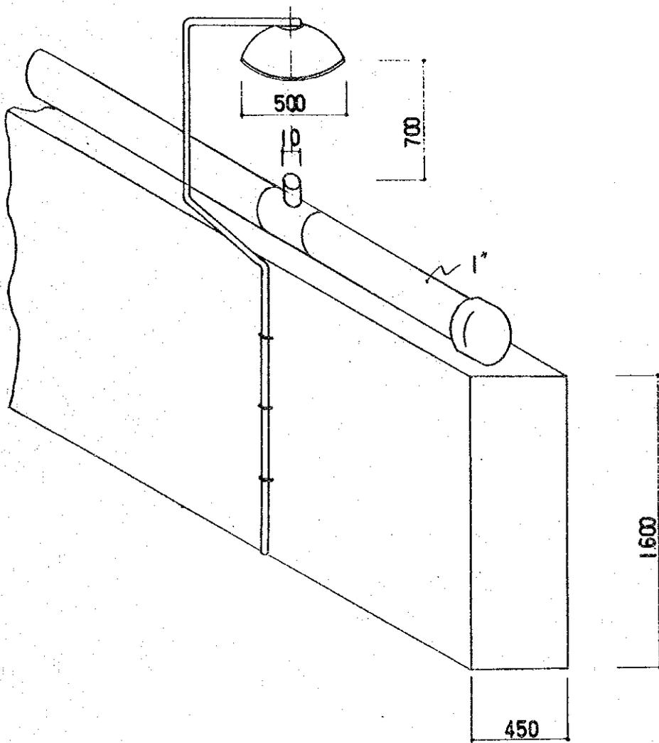
Fig. S8.4.3 Detailed sprinkler system
