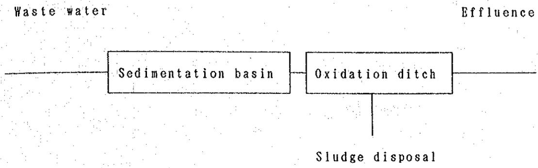
Fig.S8.5.4 One treatment method for Starch Facilities
