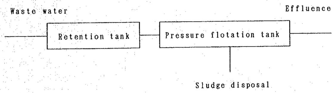
Fig.S8.5.5 One treatment method for Sorp Facilities
