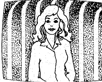
Fig. 5-10 Color lock misadjustment
