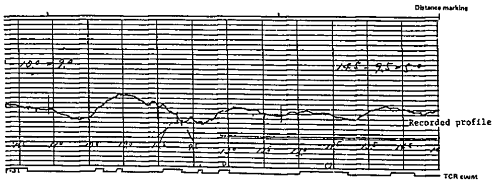
Example of Profile Recorded by 3m-Profilometer at V = 3 ~ 4 km/hr
