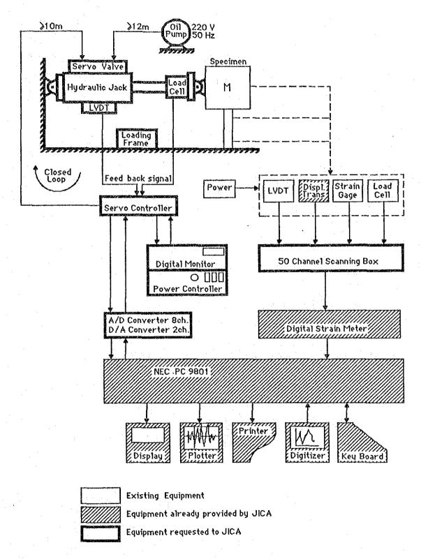
Computer Controlled Testing Equipment.
