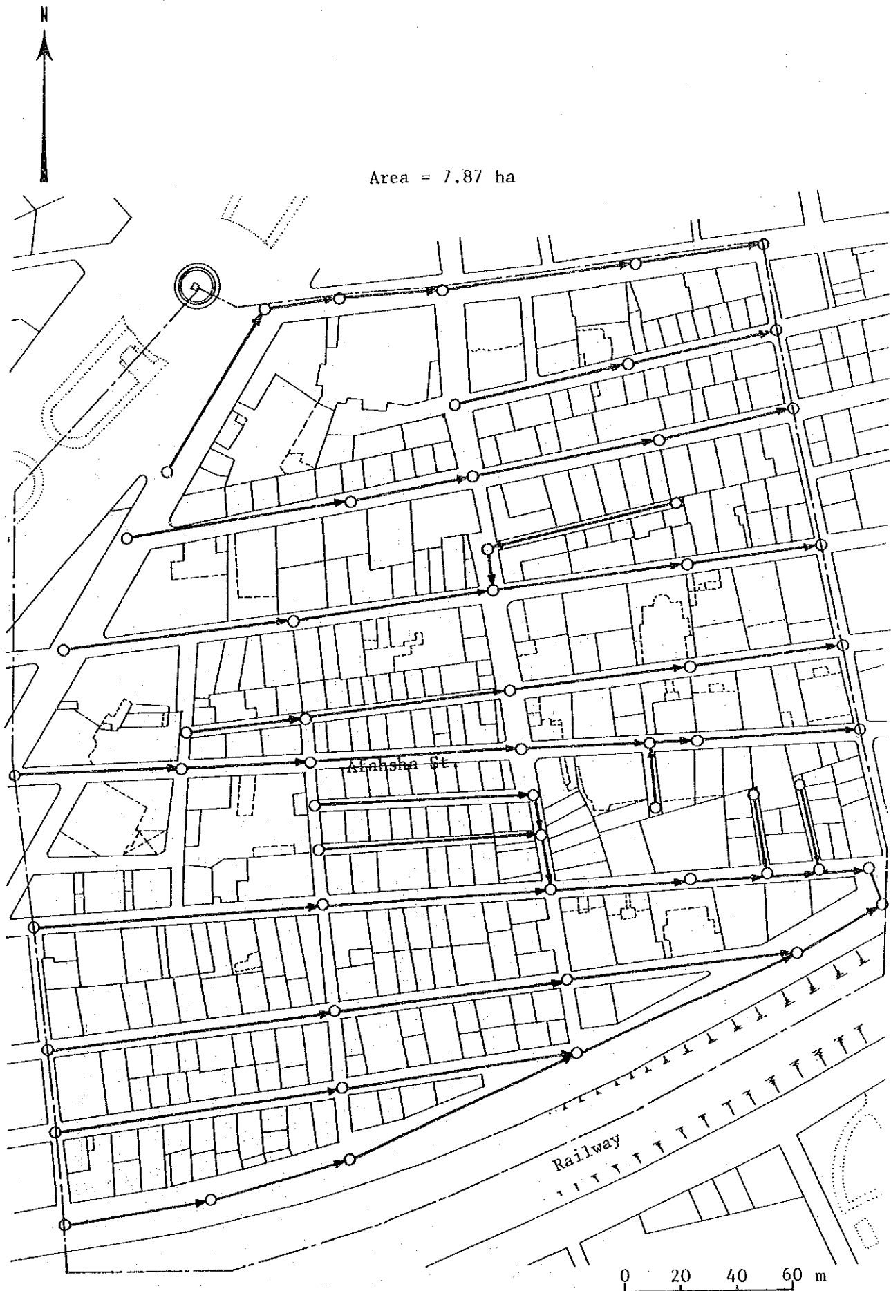
Figure VII-1 Existing Branch and Lateral Sewers in Zagazig City (Middle Class Housing Area)
