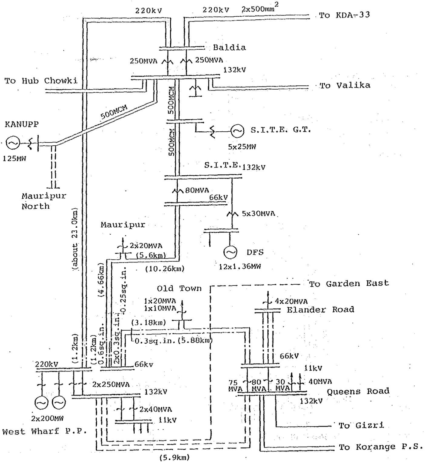
Fig.5.5-3 Transmission System Plan for West Wharf Power Plant
