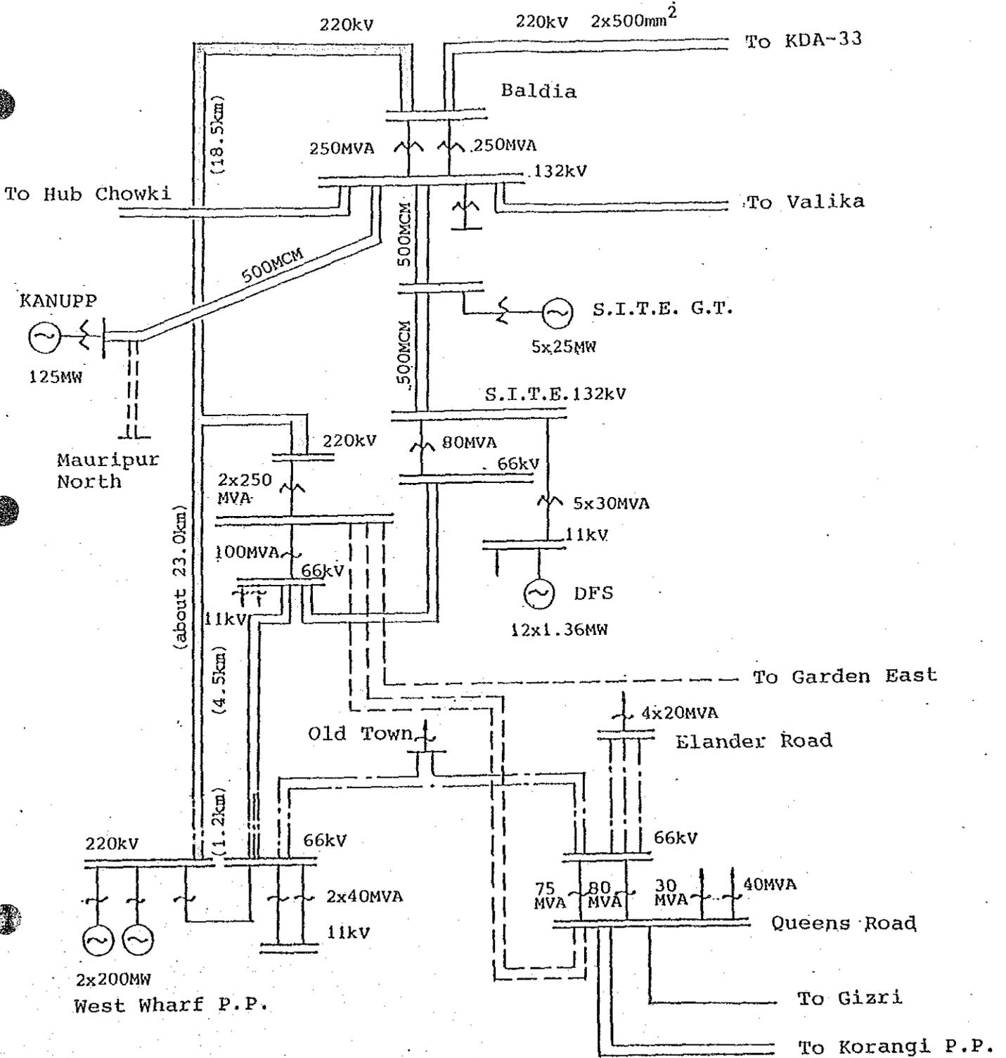
Fig. 5.5-4 Power Flow Study Diagram in 1992
