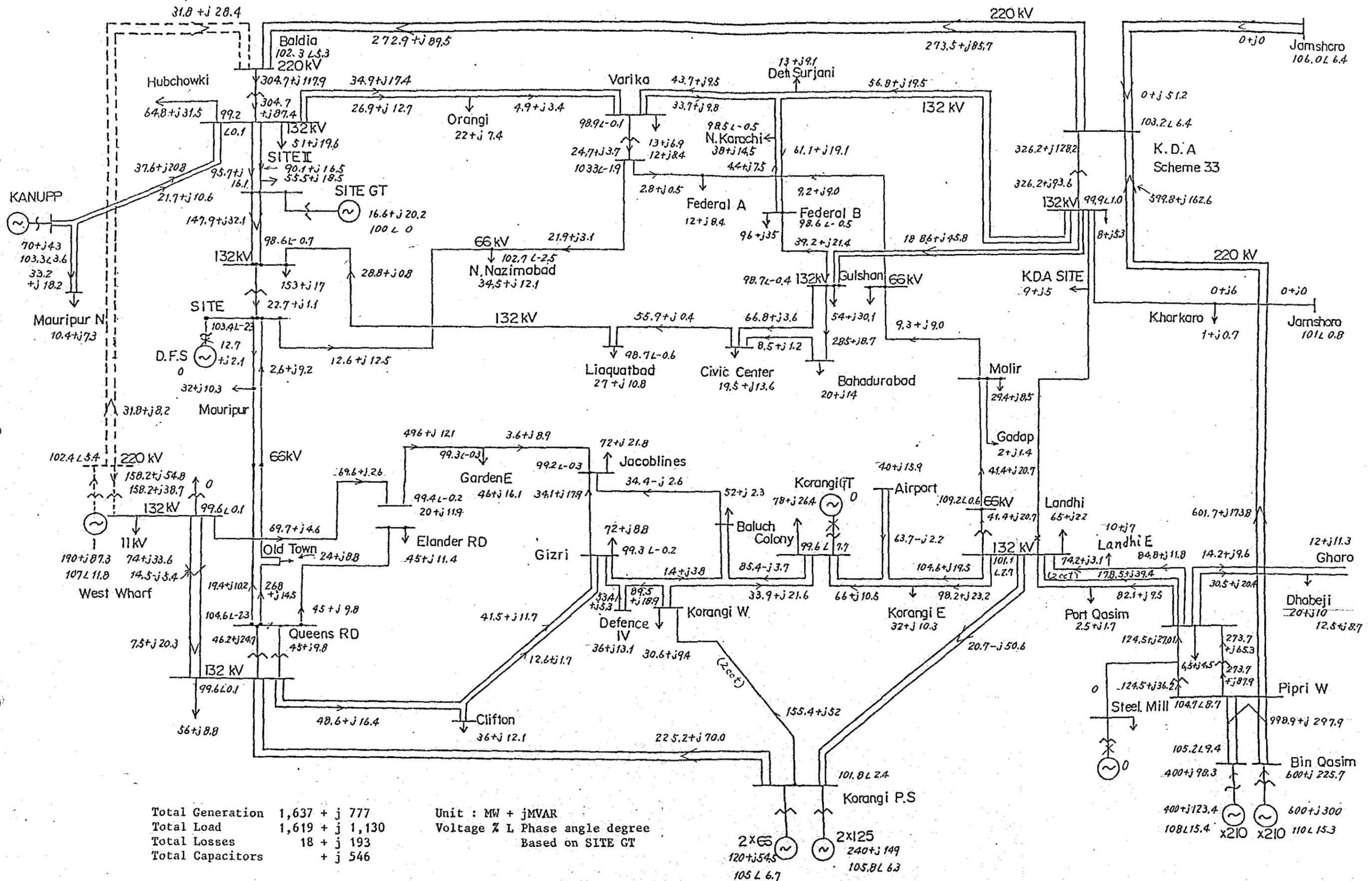
Fig. 5.5-5 Power Flow Study Diagram in 1992
