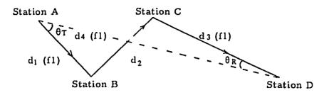
In case of the direction of Station  $C \longrightarrow Station D$  on the above diagram, Station D is influenced by the interference of undesired signal from Station A. In this case, the desired signal to undesired signal ratio (D/U) of the interference at Station D is calculated by the following equation.
