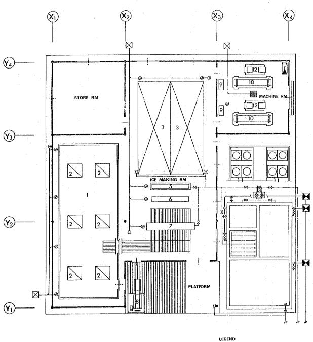
X : SOAK-AWAY E CATCH BASIN Ø : FLOOR DRAIN g : FAUCET M : VALVE P TRAW WATER PUMP ⊕ : CLEAN OUT
