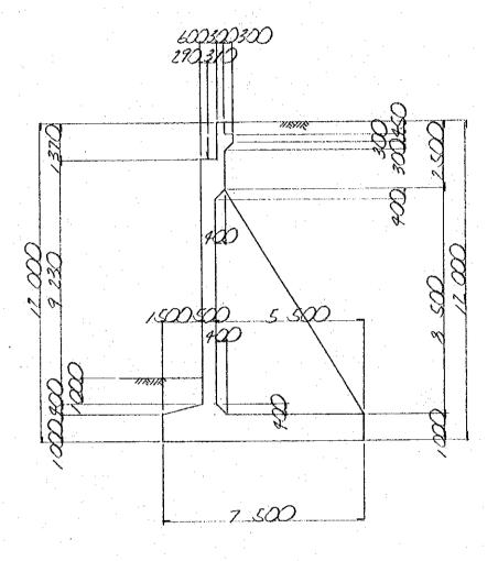
buttress span  $l = 3600^{m}$
