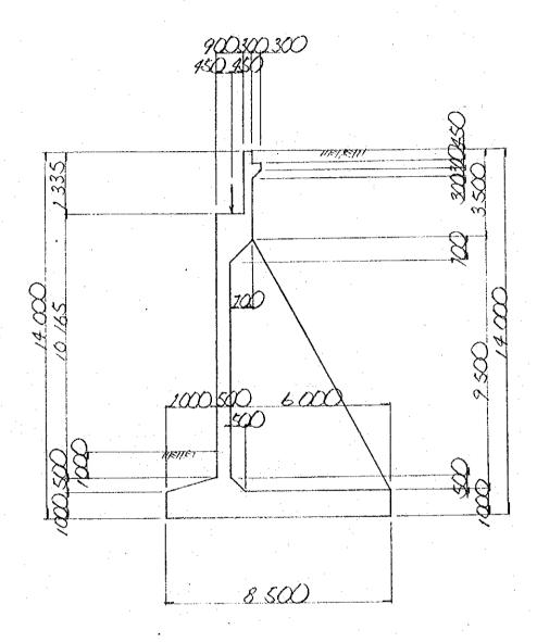
buttress span  $l = 3.100^{m}$
