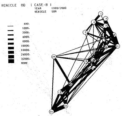
Fig. 5-6 Desire Lines for Vehicle
