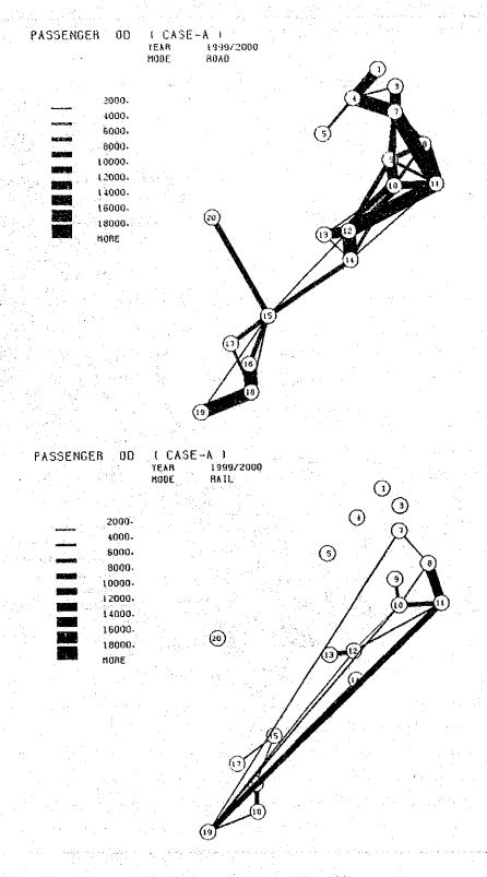
Fig. 5-2 Desire Lines for Passenger (Case A)
