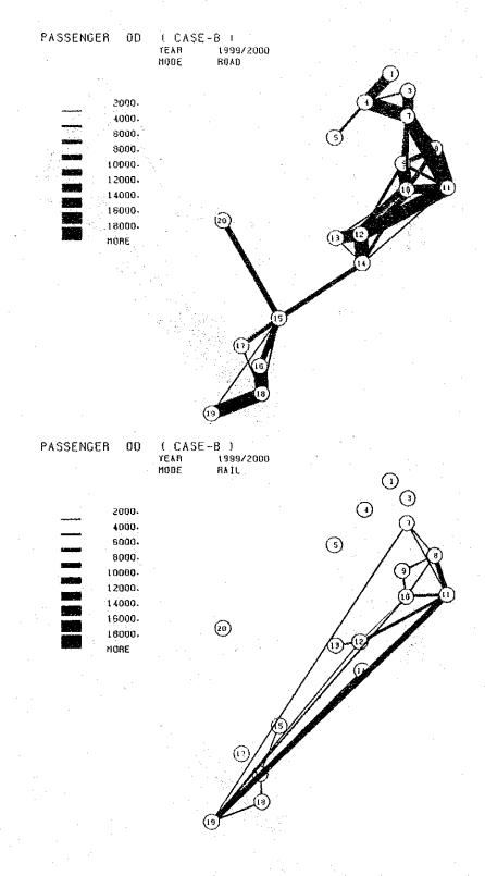
Fig. 5-3 Desire Lines for Passenger (Case B)
