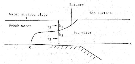
This is the rough sketch of a salt wedge. The slope bordering on the tip of the wedge and on the mouth of the river is steep while it becomes gentle in the center part.
