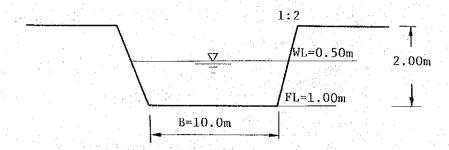
When the surface slope is 1/1000 under natural flow, the rate of discharge will be:
