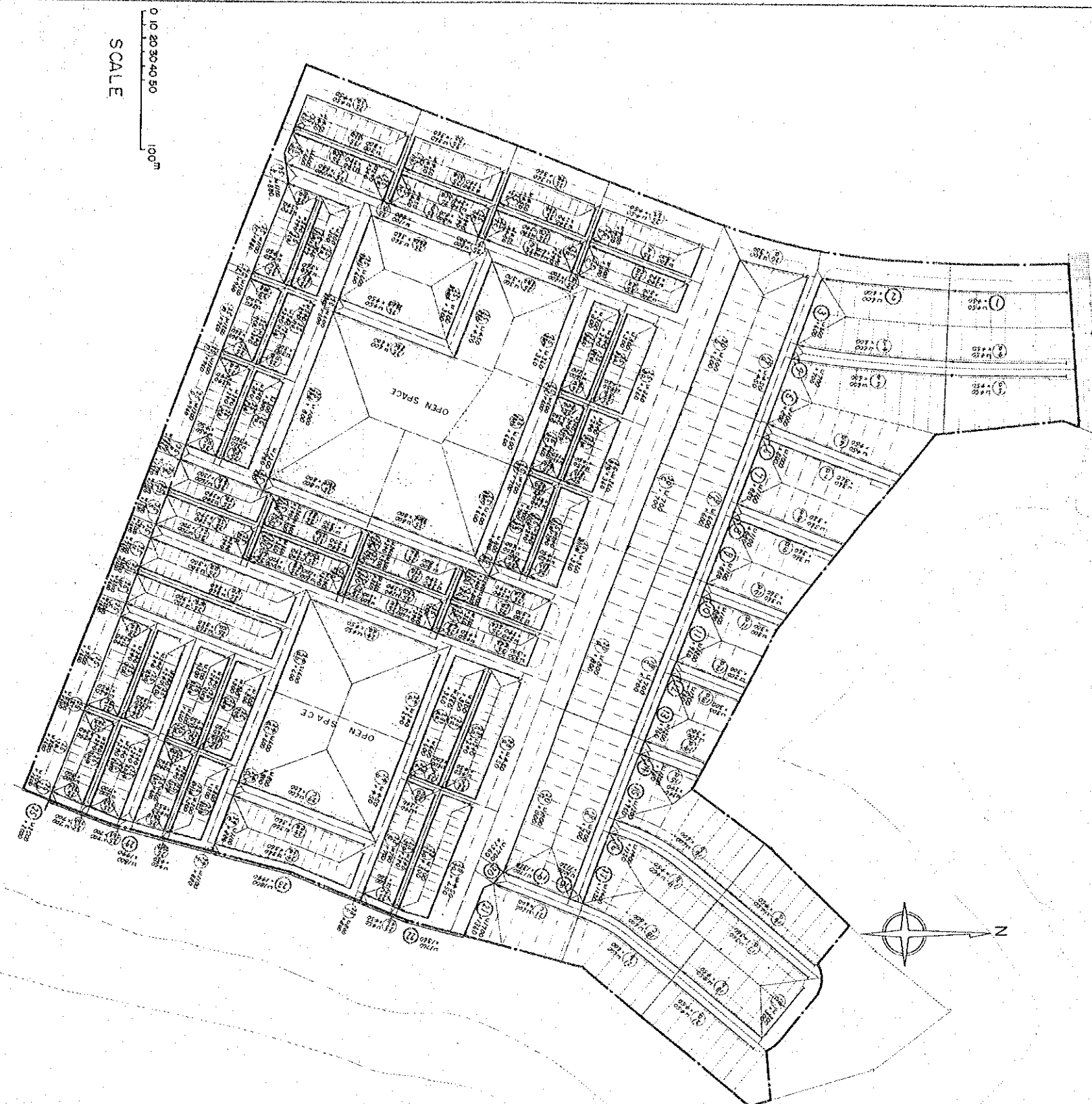
SEWERAGE AND DRAINAGE SYSTEM PROJECT BUTTERWORTH/BUKIT MERTAJAM METROPOLITAN AREA, MALAYSIA REPRESENTATIVE NETWORK OF SMALLER DRAINS IN RESIDENTIAL AREA FIGURE J - 12
