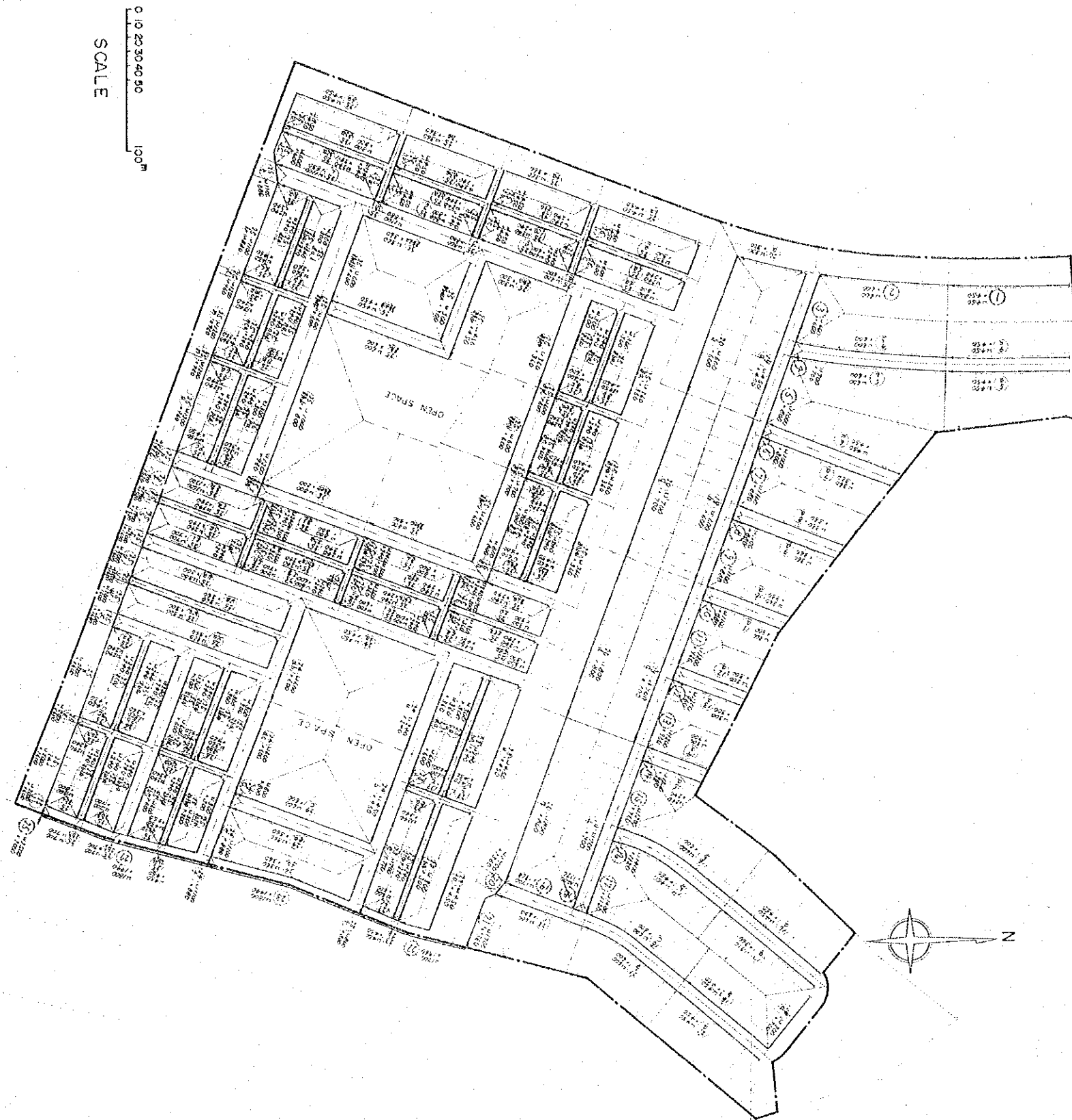
SEWERAGE AND DRAINAGE SYSTEM PROJECT BUTTERWORTH / BUKIT MERTAJAM METROPOLITAN AREA, MALAYSIA 住居地区における道路側溝網の代表例 FIGURE J-12
