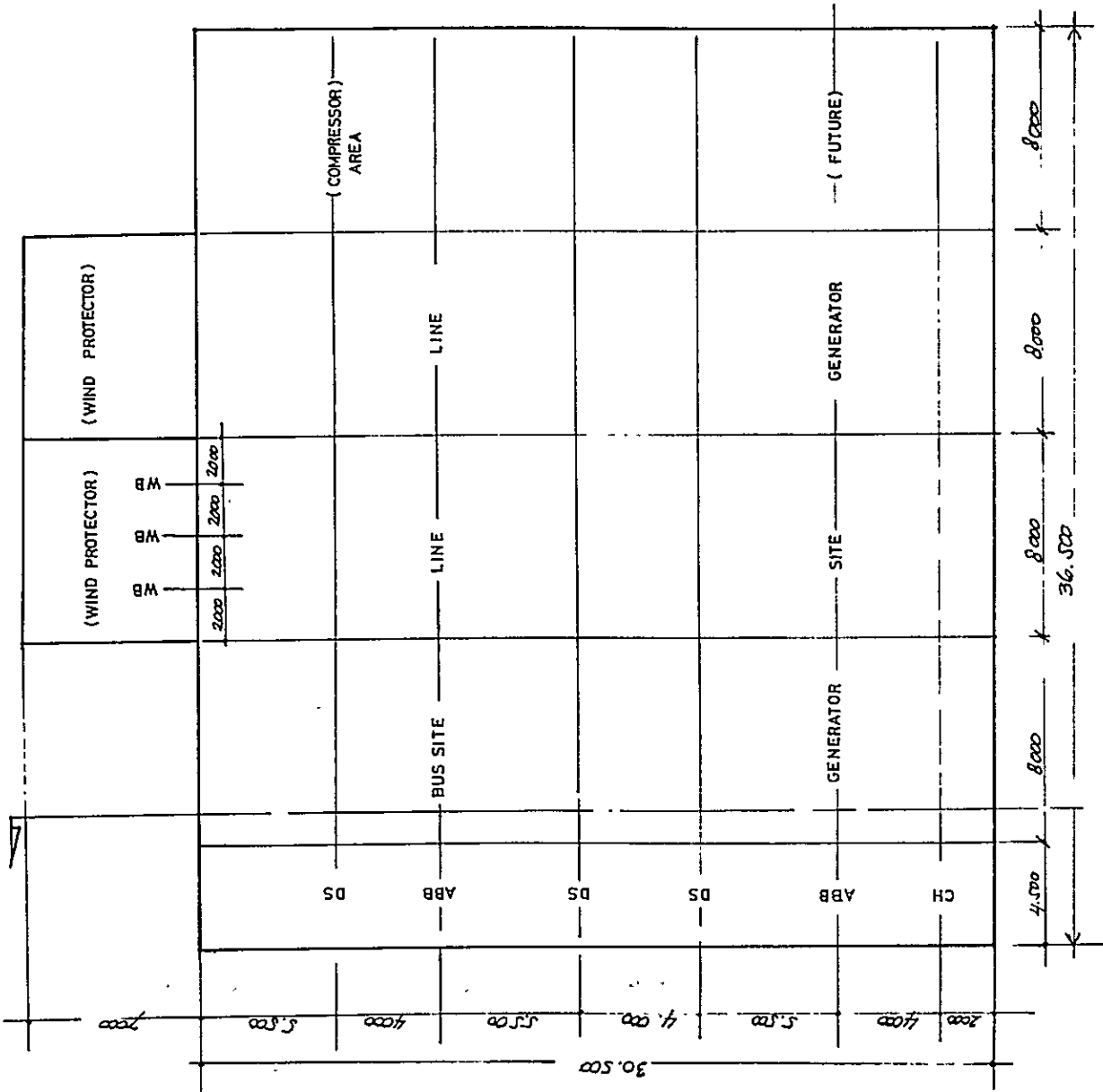
Fig. 3-2-11-(4) 150KV Indoor Switchyard with Overhead Outgoing Transmission Line
