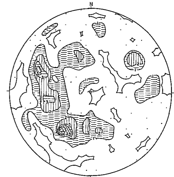
Contour Diagram of 1365 Joints which were measured at the left bank and Stereographic Projection of Major Joints (Prepared by projecting on upper semisphere)
