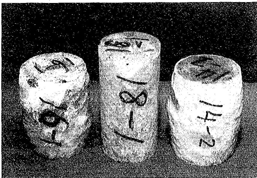
(r) Triaxial compression test. Test piece after and before testing.
